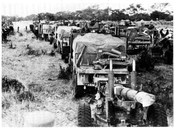
A canvas cover is supplied to cover all equipment on the cargo body. An elephant trunk-type hydraulic crane is mounted behind the rear cargo body, capable of swinging through 360 degrees and lifting 800 kg at a jub length of 3,5 m. The overall dimensions of the vehicle are 2,5 m wide  $\times$  9,35 m long  $\times$  3,35 m high.
