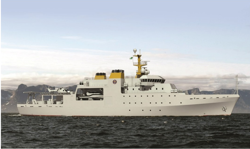
Figure 6: An artist's impression of the new hydrographic survey vessel of the SAN, currently being built in Durban as part of Project Hotel. A pennant number A187 has been allocated, while the ship will be named SAS Nelson Mandela. An ice-strengthened bow and the ability to carry a Westland Lynx helicopter will make it suitable to carry out expeditionary operations in the Southern Ocean. 122
